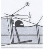
An extension may not be used to provide the 50 mm space between the ROPS and the Competitors/Drivers helmet.
